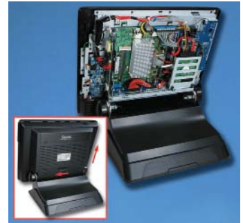
Tool-Free Access to RAM, Hard Disk Drive and Compact Flash Card Optimizes Serviceability
